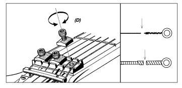
In the case of TRS101 tremolo, replace the strings one by one. Removing all the old strings at once will release the tension on the tremolo and change the tremolo angle "up-pull."
