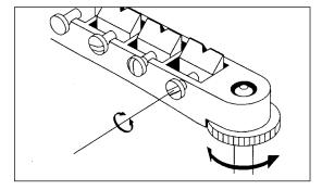
To replace strings, thread the new strings through the string holes located on the back of the tailpiece and bring them up and over the saddle. The intonation can be adjusted by moving the saddle forward or backward using a Slot head (-) screwdriver on the adjustment screw at the rear of the bridge. String height is controlled by raising or lowering the two height adjustment spinners on either side of the bridge. The height adjustment of
