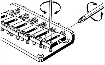
To change strings, thread the new strings through the string grommets located on the back of the guitar and bring them up and over the saddle. The intonation can be adjusted by adjusting the saddle forward or backward using a Phillips (+) head screwdriver on the intonation adjustment screw at the rear of the bridge. String height is controlled by raising or lowering the small Allen screws using a wrench on either side of the saddle.
