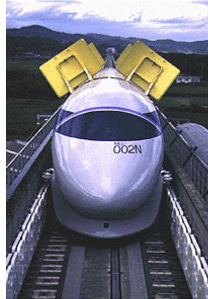
**Figure 4. Yamanashi MLU002N with aerodynamic brakes deployed [13]**
