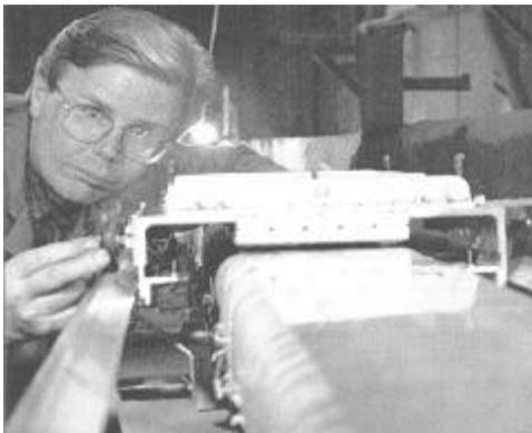
**Figure 8. Inductrac test model on its guideway at the Lawrence Livermore National Laboratory [18, p. 71]**
