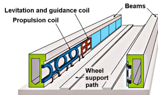
**Figure 6. Yamanashi beam method of guideway construction [13]**
