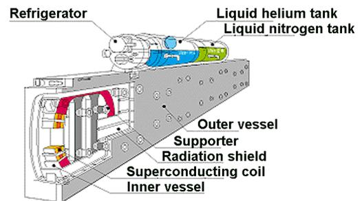
**Figure 3. Yamanashi Superconducting Magnet [13]**
