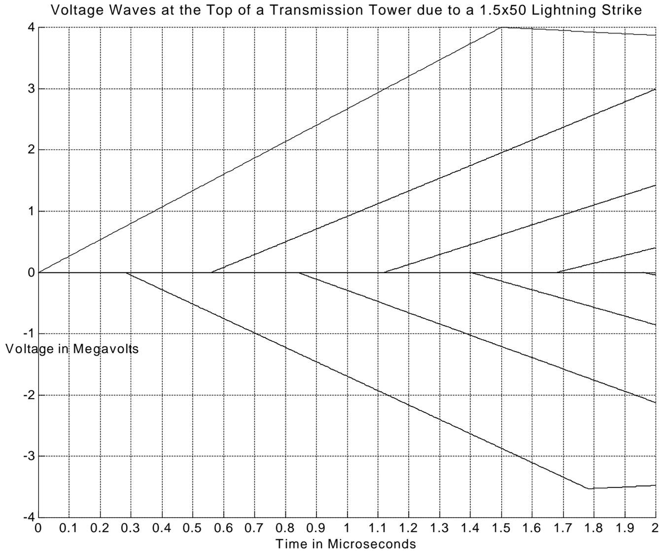
Note that each plot shown except for the initial wave (the initial wave intersects the origin) represents 2 plots superimposed, an upward traveling wave and its equal downward reflection.
