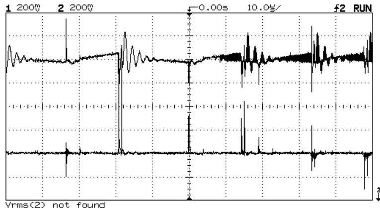
Input voltage (upper trace) and output voltage (lower trace) as seen on our experimental circuit board setup. Voltage ripples at the input appear to be associated with the 30 kHz clock frequency (period =  $33.3 \mu s$ ). Spikes at the output are more random with values up to about  $1 V_{pp}$ .
