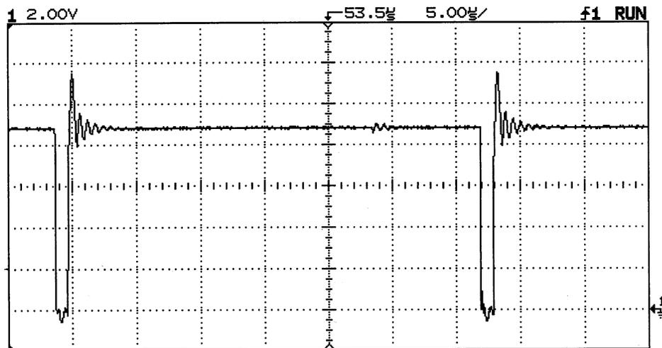
**30KHz square wave oscillator output**
