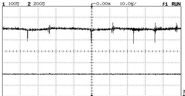
Input voltage (upper trace) and output voltage (lower trace) after adding the 820  $\mu\text{H}$  inductor and 470  $\mu\text{F}$  capacitor at the output. Output noise, which is on the 100 mV per division scale (the smallest scale available on this equipment for a 25-volt signal), is barely perceptible, less than 10  $\text{mV}_{\text{pp}}$ , which is less than the 20 mV maximum specification.
