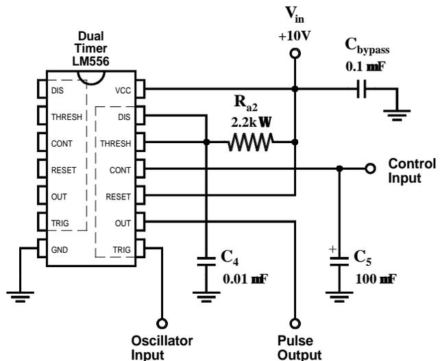
**Pulse Width Modulator Circuit**
