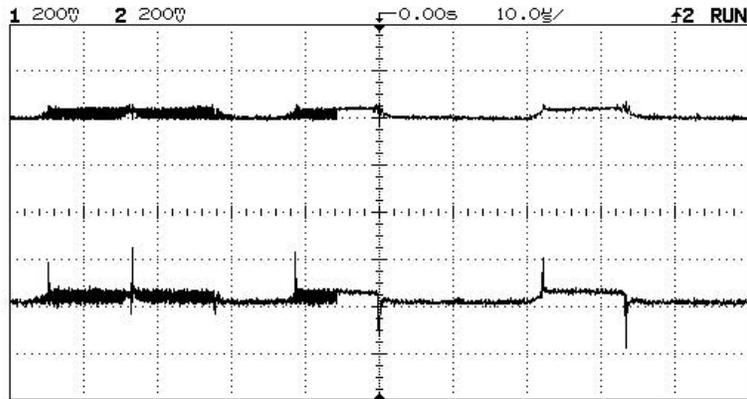
Input voltage (upper trace) and output voltage (lower trace) before adding the 820  $\mu\text{H}$  inductor and 470  $\mu\text{F}$  capacitor at the output. Output noise appears to be about 400  $\text{mV}_{\text{pp}}$ , substantially more than the 20 mV we are looking for.
