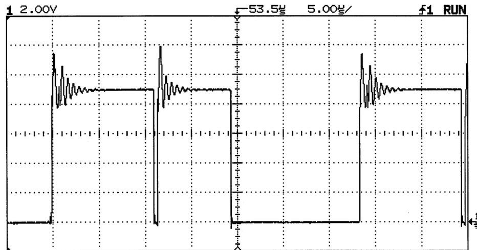
**Splitting of the pulse from the pulse width modulator**
