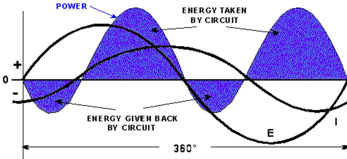
**Figure C. Power Cycle with an Inductive Device**
