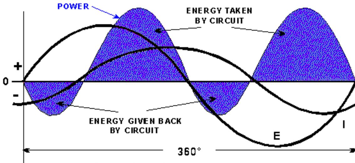
**Figure C. Power Cycle with an Inductive Device**
