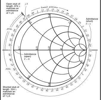
In this example, all values were in units of admittance. If we were interested in finding a stub length for a series stub problem, the units would be in impedance. The problem would be worked in exactly the same way. Of course in impedance, an open shunt (zero length) would have the value  $Z=\infty$ , representing a point at the right end of the x-axis.
