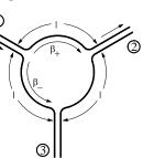
Port 3 is terminated internally by a matched load. With a source at 1 and a load at 2, any power reflected at the load is absorbed by the load resistance at port 3. A 3-port network cannot be both lossless and reciprocal, so the circulator is not reciprocal.
