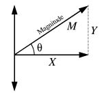
In the descriptions above, impedance is used as an example. Rectangular and Polar Notation can also be used to express amperage, voltage, and power.
