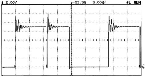
Splitting of the pulse from the pulse width modulator
