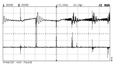
Input voltage (upper trace) and output voltage (lower trace) as seen on our experimental circuit board setup. Voltage ripples at the input appear to be associated with the 30 kHz clock frequency (period =  $33.3 \,\mu$ s). Spikes at the output are more random with values up to about 1 V<sub>pp</sub>.
