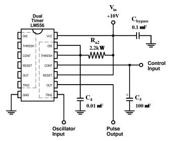
**Pulse Width Modulator Circuit**
