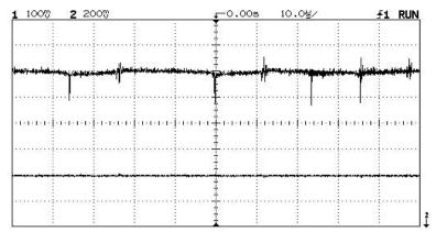
Input voltage (upper trace) and output voltage (lower trace) after adding the 820  $\mu$ H inductor and 470  $\mu$ F capacitor at the output. Output noise, which is on the 100 mV per division scale (the smallest scale available on this equipment for a 25-volt signal), is barely perceptible, less than 10 mV<sub>pp</sub>, which is less than the 20 mV maximum specification.
