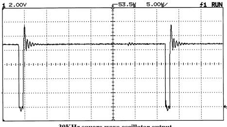
30KHz square wave oscillator output
