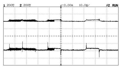
Input voltage (upper trace) and output voltage (lower trace) before adding the 820  $\mu$ H inductor and 470  $\mu$ F capacitor at the output. Output noise appears to be about 400 mV<sub>pp</sub>, substantially more than the 20 mV we are looking for.
