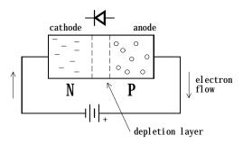
An <u>ideal diode</u> acts like a closed switch when forward biased and an open switch when reverse biased. <u>1st</u> <u>approximation</u> calculations assume an ideal diode. <u>2nd approximation</u> calculations take into account the voltage drop across the diode. <u>3rd approximation</u> calculations additionally take into account bulk resistance.
