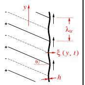
Particle displacement:  $\xi(y,t) = e^{j\omega(t-y/C_p)}$
