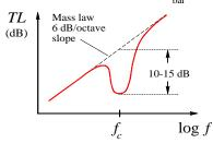
**Design considerations:** If  $f < f_c$ , use the diffuse field mass law to find the transmission loss. If  $f > f_c$ , redesign to avoid. Note that  $f_c$  is proportional to the inverse of the thickness.
